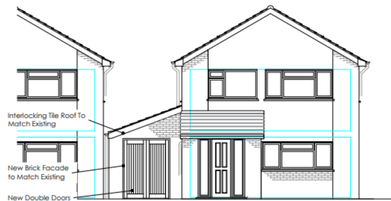
PROPOSED SOUTH ELEVATION 1:50
